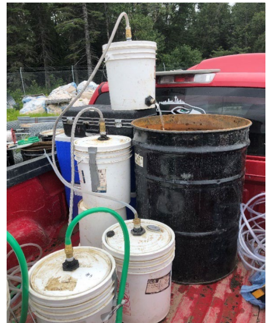
Exhibit 2-5: Filtering purge water with GAC
